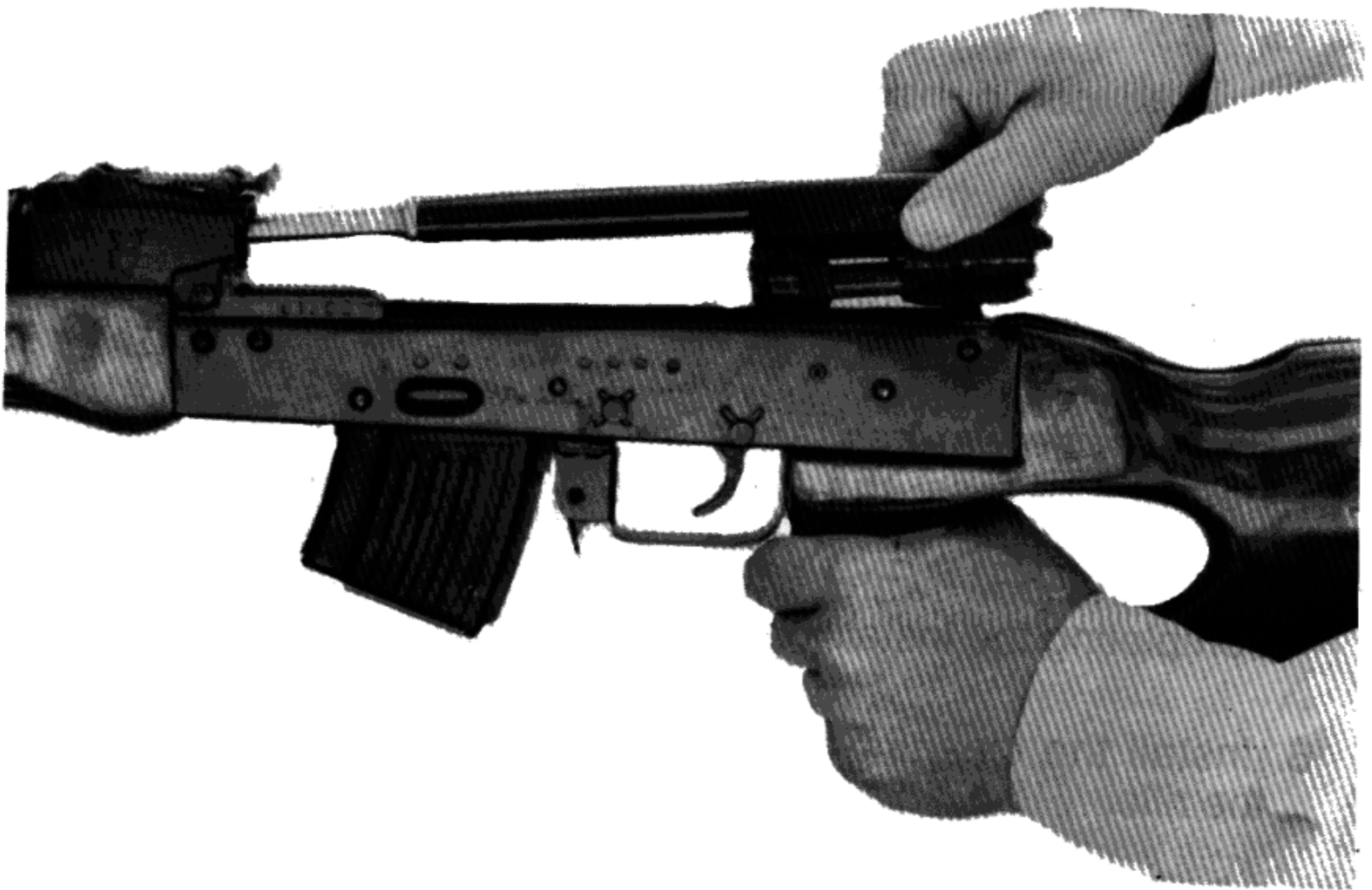
FIG. 11 ATTACHING THE BOLT CARRIER WITH THE BOLT TO THE RECEIVER
