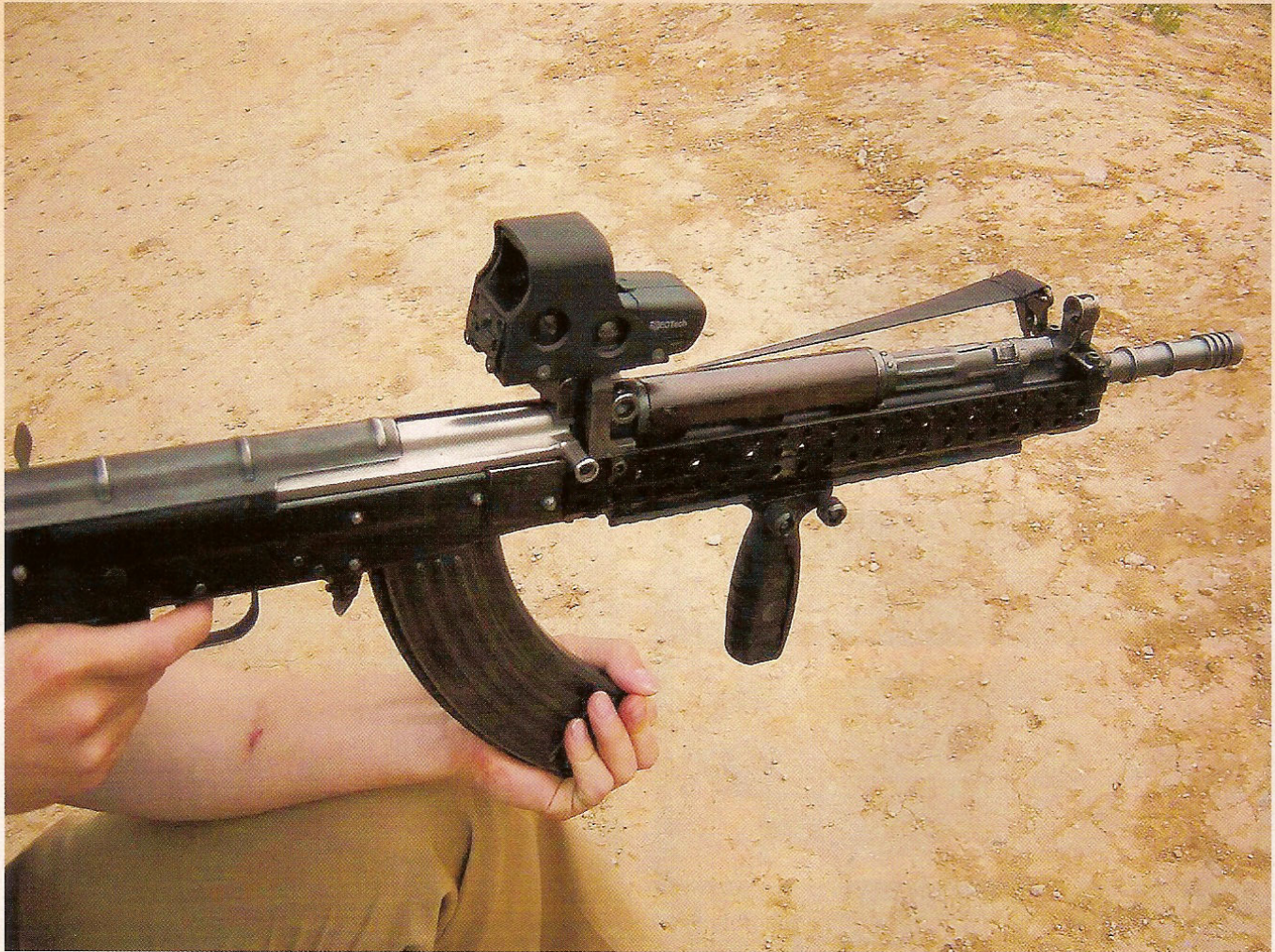
The aftermarket rail forehand guard provides three long rails and one short one on top for mounting optics like the EOTech seen here.
