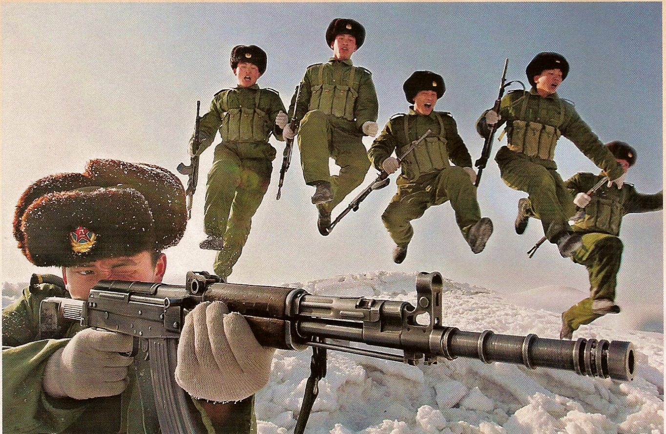
A PR image from the Chinese army. The front sight of the Type 81 was moved back to make room for the rifle-grenade adapter.
