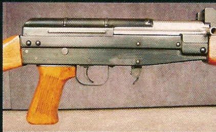
Both the rifle and light machine gun use the same receiver, rated for a 20,000-round service life. The latitudinal bend in the middle of the receiver helps to stiffen it. Photo courtesy of Craig Adams
