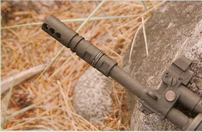
The Rk 95 TP features a combination muzzlebrake/grenade launcher, which also accepts a sound suppressor.
