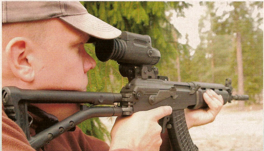
One drawback to side-mounted optics is that they tend to sit rather high.
