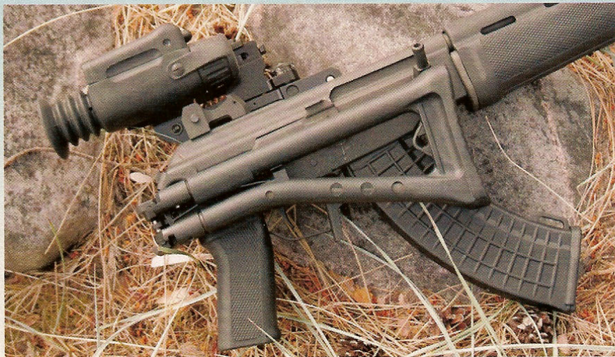
The stock folds to the right to prevent it from interfering with side-mounted optics.
