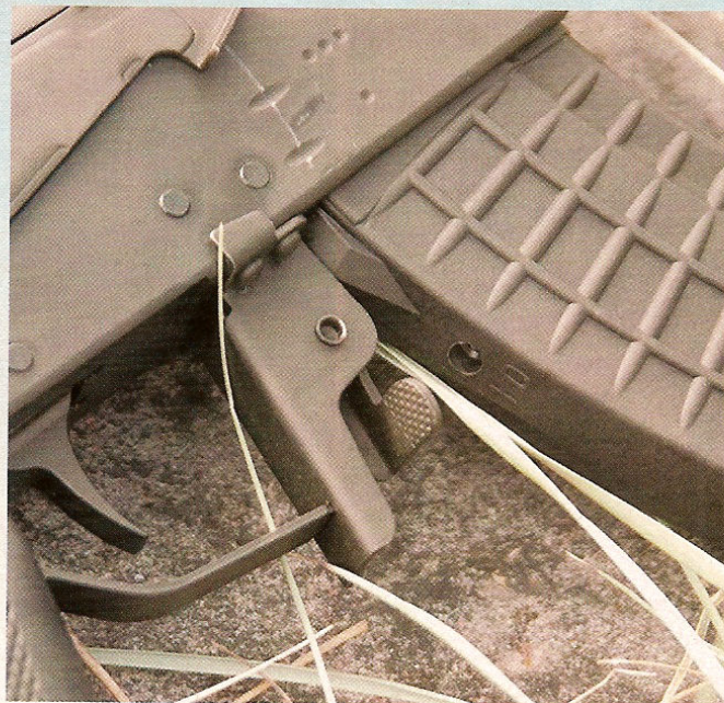
The Rk 95 TP's magazine release is an extended paddle.
