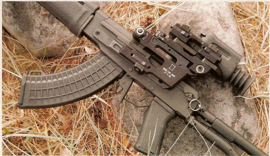
A side rail allows day/night optics to be easily mounted. Also note the top-cover retainer.
