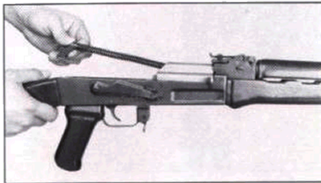
Fig. 27 Pulling the recoil spring assembly out of the bolt carrier.
