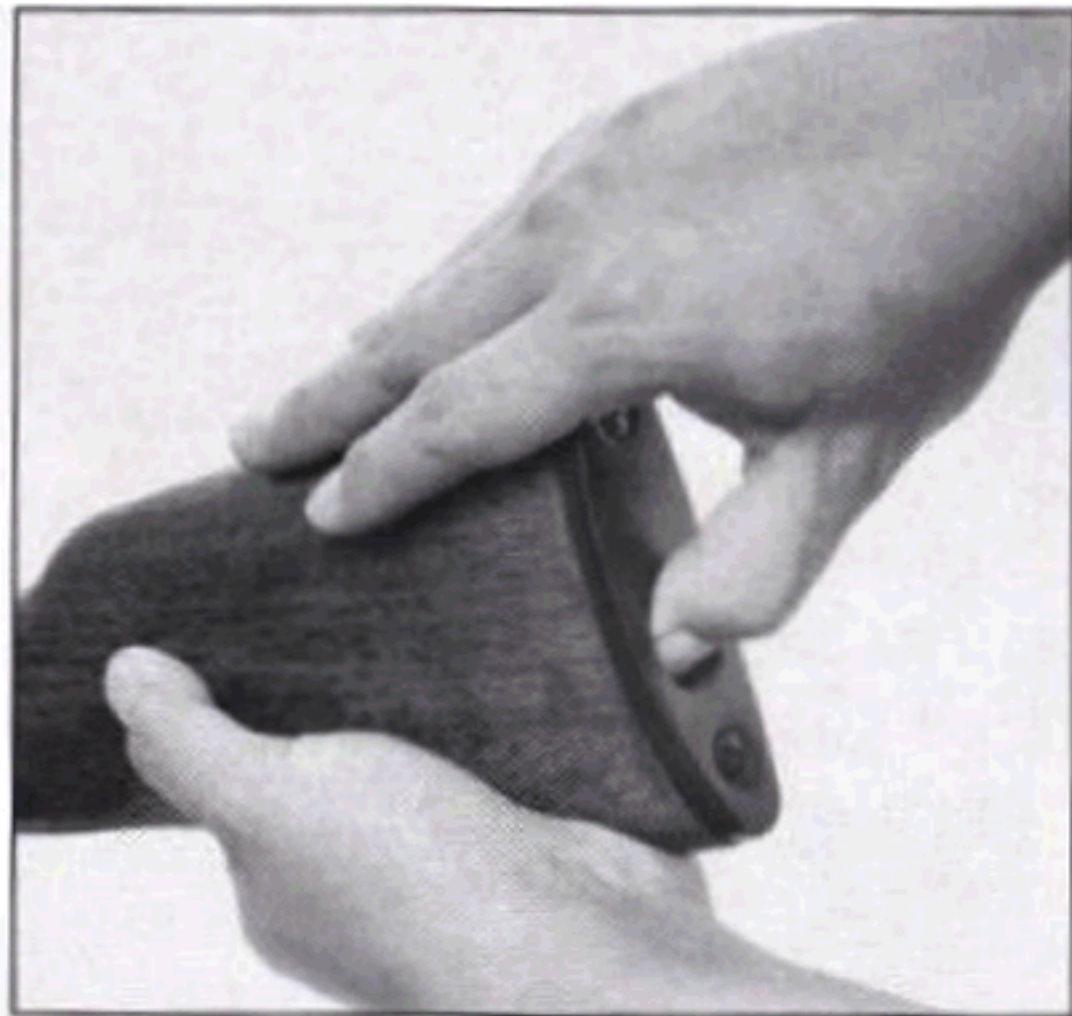
Fig. 34 Depress the spring-loaded trapdoor.
