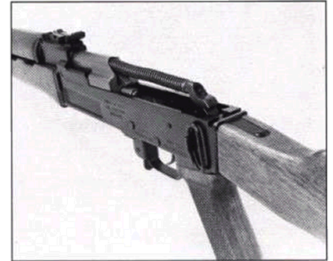
Fig. 33 The recoil spring guide placed forward and under its slot during reassembly.
