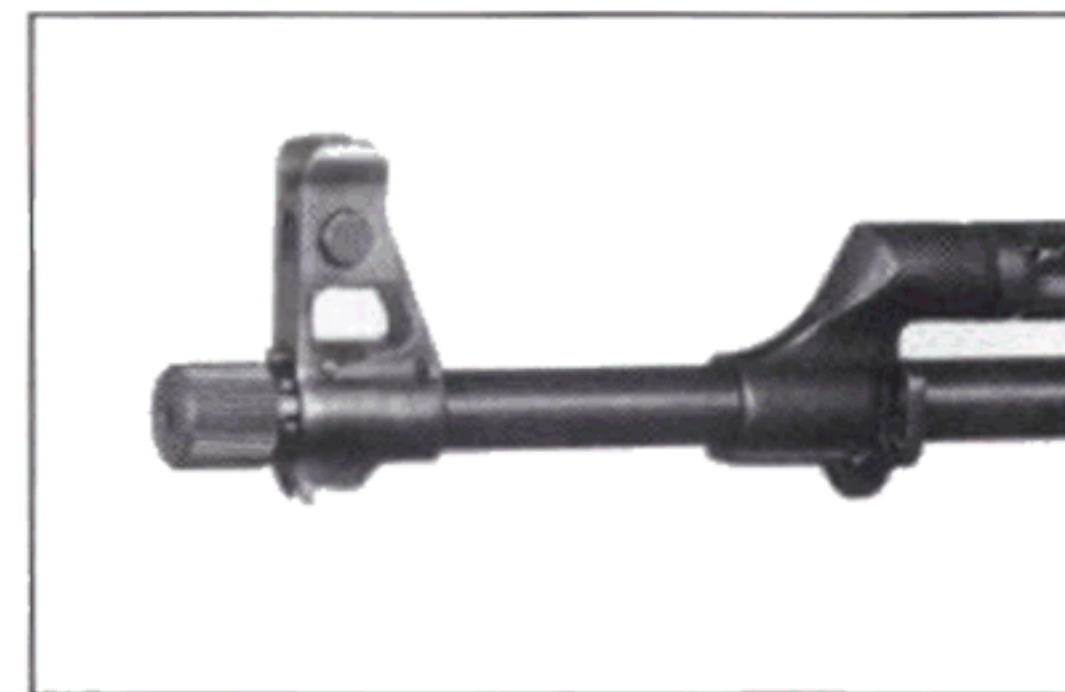
Fig. 18 Rifle with the blank firing device installed.
