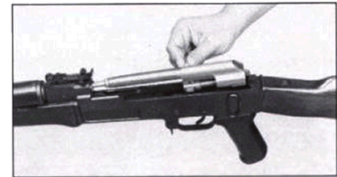
Fig. 28 Pulling the bolt carrier/gas piston out of the receiver.
