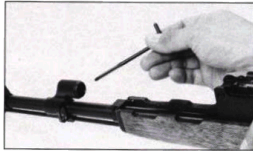
Fig. 38 Insert the squared end of the residue scraper into the gas port.
