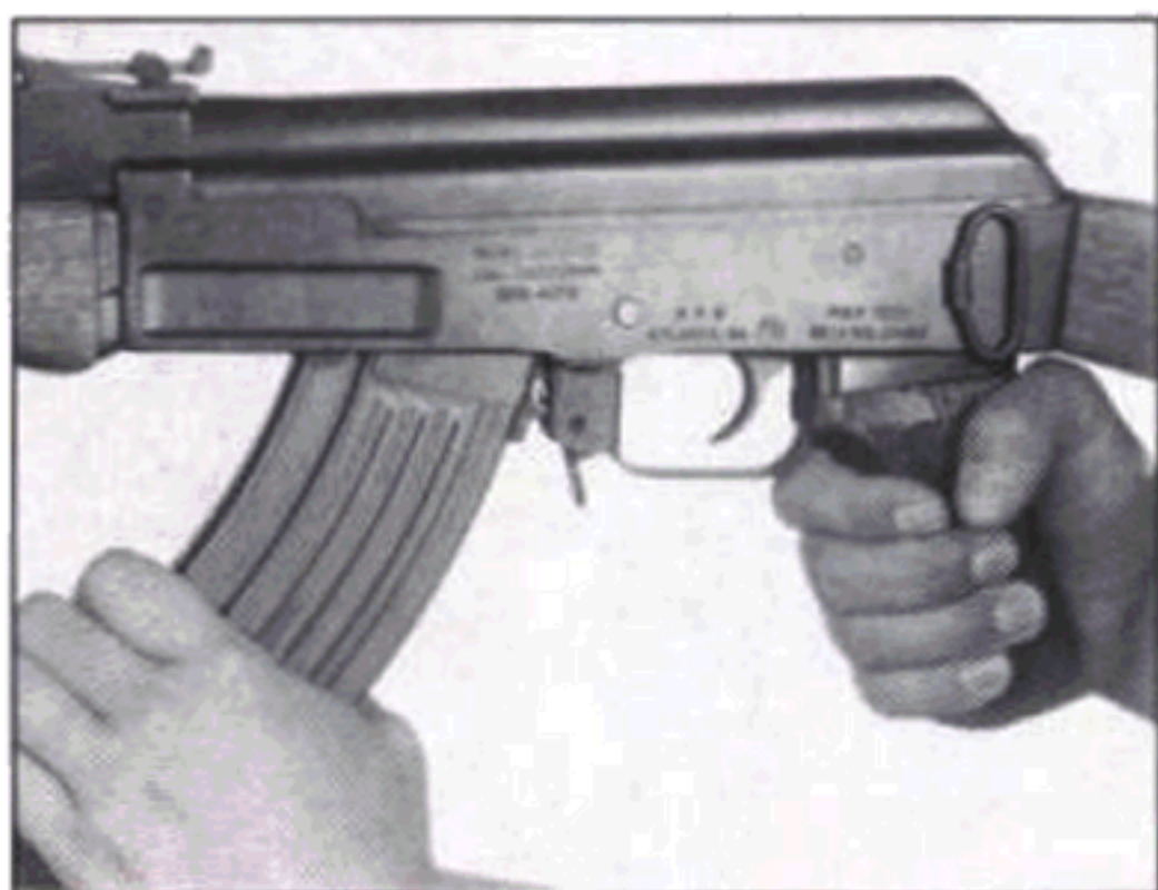
Fig. 13 Inserting the magazine.
