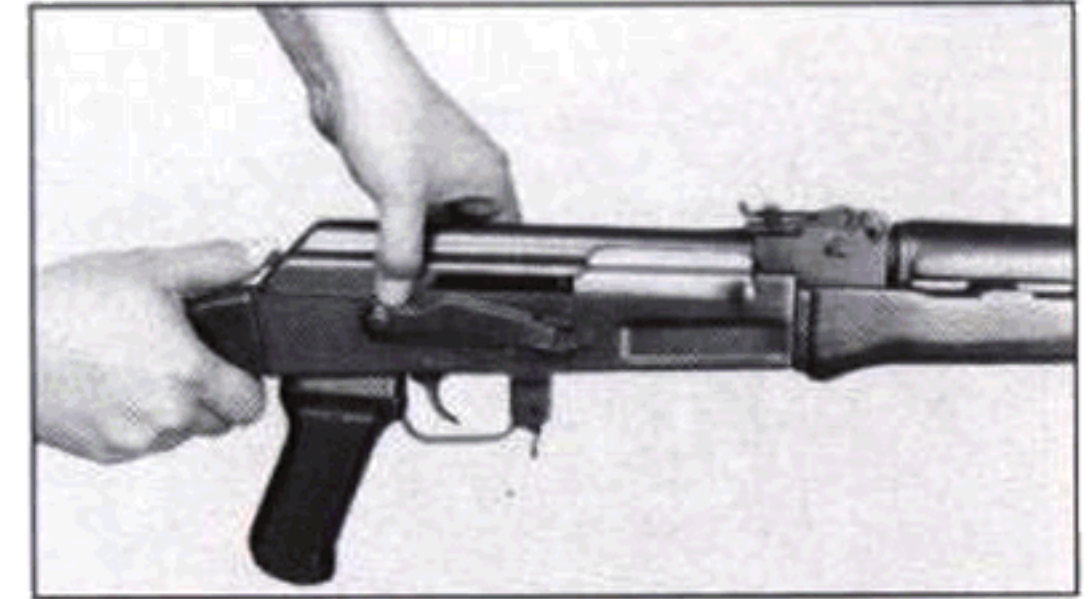
Fig. 25 Push in the serrated tip of the recoil spring guide . . .
