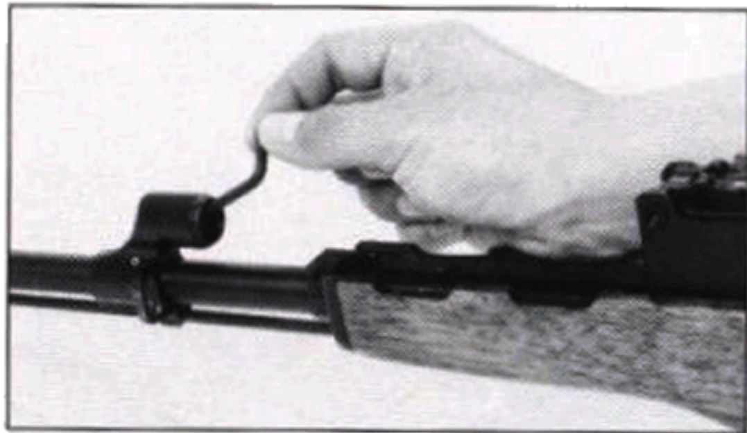
Fig. 39 Turn the residue scraper until fouling is removed.
