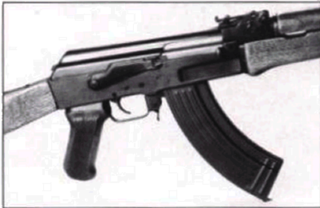
Fig. 8 The safety lever in the "SAFE" position.
