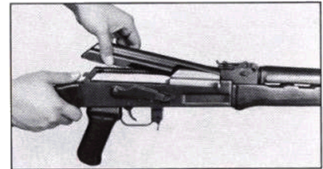
Fig. 26 . . . lift the receiver cover off.
