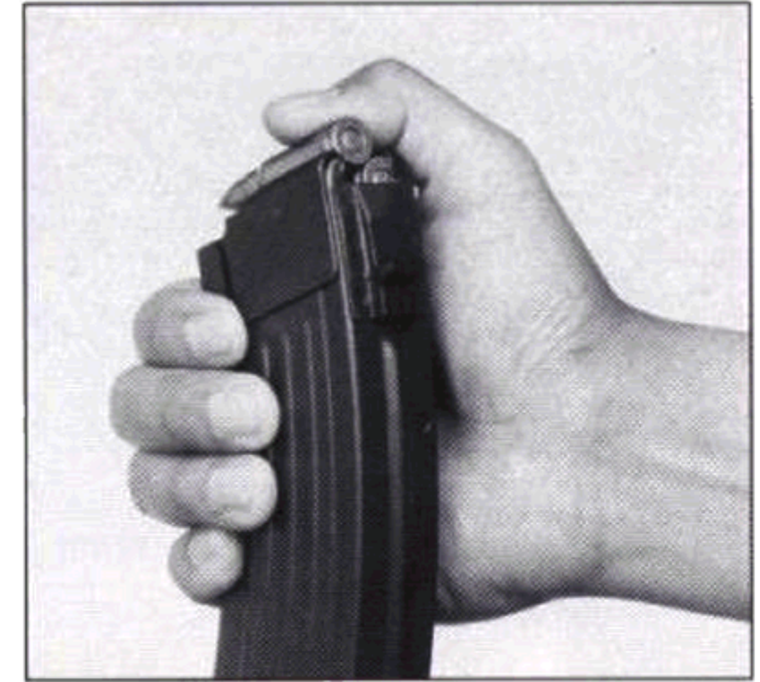
Fig. 10 Loading the magazine.
