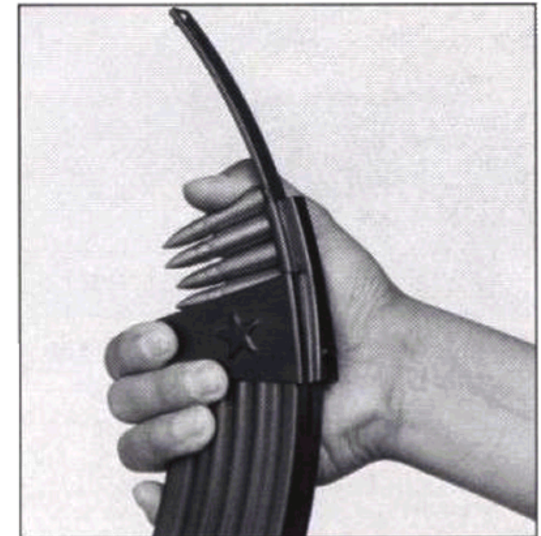
Fig. 11 Loading the magazine using the quick-loading tool and ammo on 10-round stripper clips.
