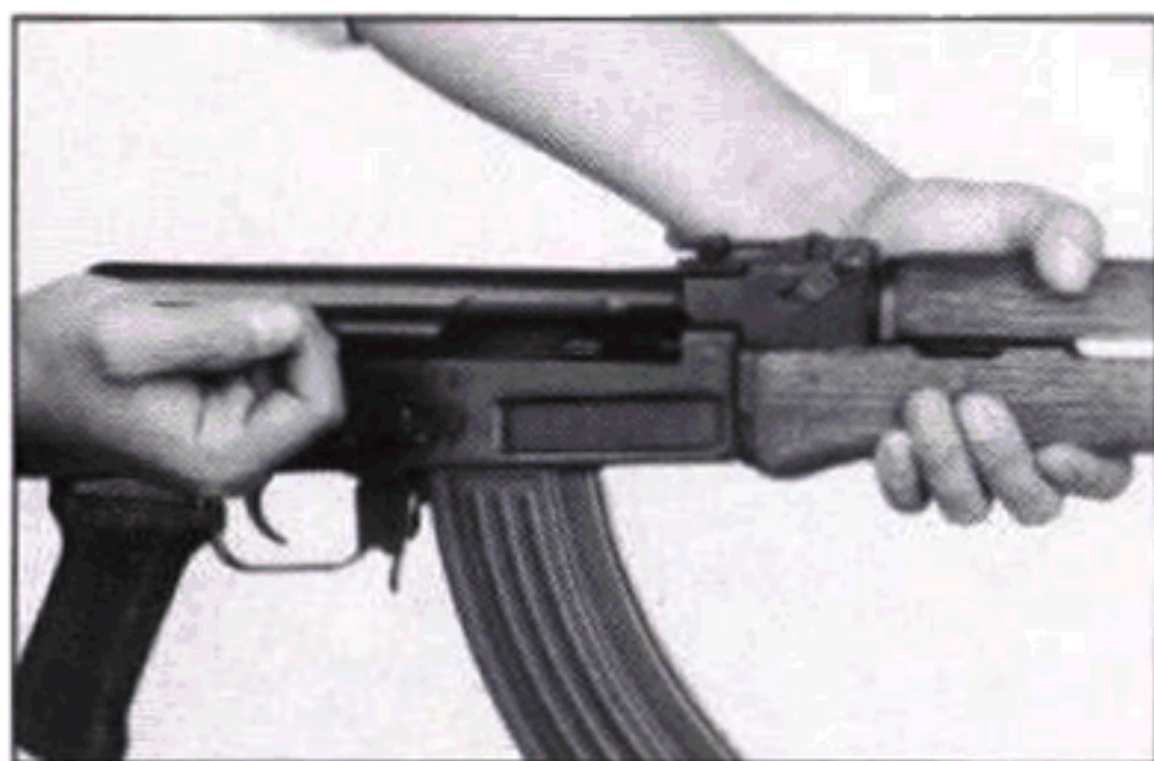
Fig. 14 Chambering a round in the rifle (Note that the fingers are kept away from the trigger guard).
