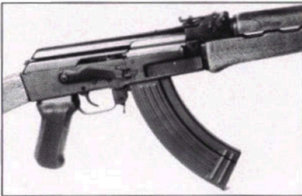
Fig. 9 The safety lever in the "FIRE" position.
