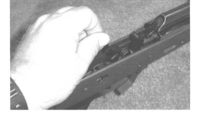
When routing the plate forward, ensure that the open end of the plate is secured in the groove of the hammer pin, between the receiver wall and the hammer spring. It may be necessary to "push" the coils of the hammer spring out of the way in order to seat the hammer pin. Push the plate forward until Area A is securely around the hammer pin and positioned in the groove of the pin.
