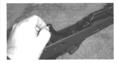
Place the retainer plate such that the open end (Area A) is forward, and slide it along the opposite side of the receiver from where the selector would be positioned. The closed circle and tail of the plate (Area C) will be positioned toward the rear of the rifle, as the selector yoke will ultimately be routed through the closed circle in the retainer plate.
