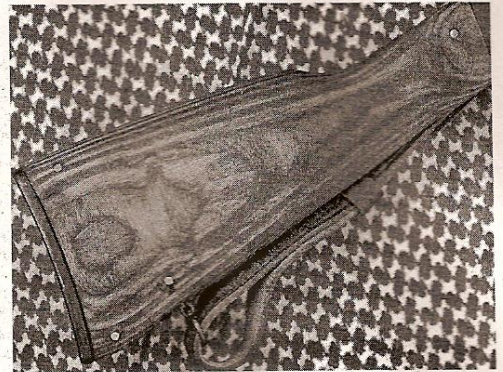
The fixed buttstock on this Romanian AKM is made of laminated beech, reinforced with steel pins. Kokalis prefers a fixed stock, saying it makes for a sturdier hold.
