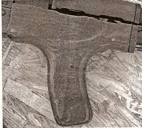
This slightly forward-sloping pistol grip forearm was made from a single piece of laminated beechwood. The slanted grip allowed the bottom-folder stock to close.
