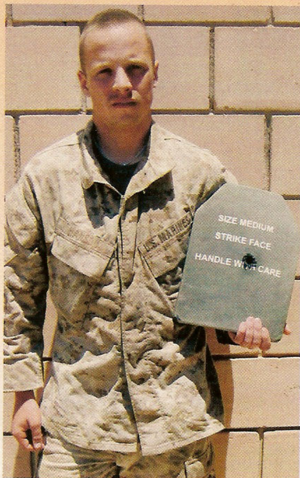
Despite making a good shot, a sniper failed to kill Marine Pfc. Joshua Hanson when his 7.62mm bullet was stopped by Hanson's SAPI plate. Photo courtesy of the USMC
