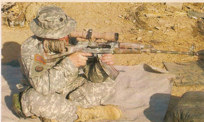
Another sniper rifle fielded by the insurgents is the 7.62x39mm Tabuk. Built in Iraq with Serb assistance, it is a simple DMR based upon the RPK. Photo courtesy of LTC Kendrick McCormick
